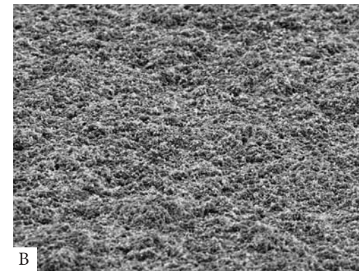
FIGURE 10-2 A, Titanium plasma-sprayed surface at high magnification. B, Acid-etched titanium surface at low magnification. C, Hydroxylapatite-coated surface at low magnification.
