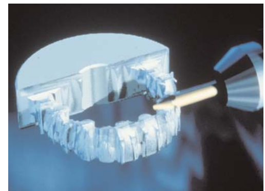
FIGURE 13-51 By entering scanning information into a computer bank, computerized lathes with precisely controlled cutting heads attack the titanium blank to create the milled bar structure.
